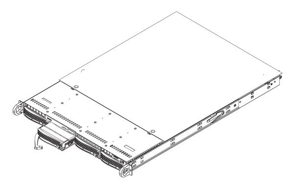
Figure 6-5. Removing a SATA Drive from the Server
